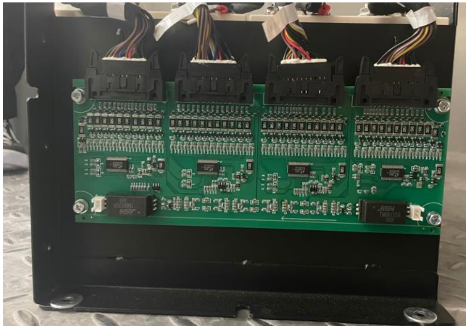
Front view of PCB for Slave Board
